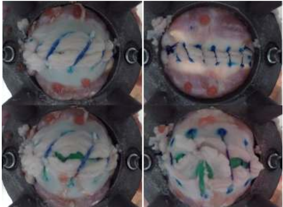
Fig. 3 Screen captures of 0 DuraMesh (left) and 1 PDS double-loop (right) laparotomy closure failure via ball-burst apparatus. The tissue sample is circumscribed by the black ring, and the ball-burst piston is colored in green, pushing through the sutured section of the sample. Top row shows samples prior to pull-through, and bottom row illustrates examples of pull-through
