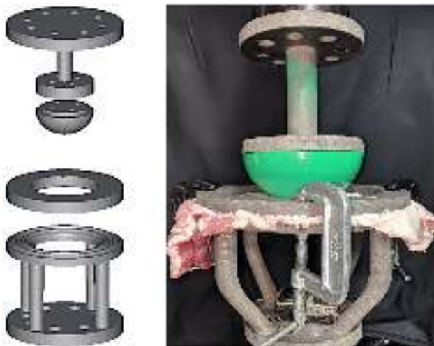
Fig. 2 Ball-burst Apparatus—Right—3D printed titanium with plastic head colored green. Upper portion includes spherical head attached to piston in order to apply force to the sample being held in the ring below. Left: computer-aided design (CAD) image of ball-burst apparatus. Ring diameter of ball-burst apparatus is 7 cm (color figure online)
